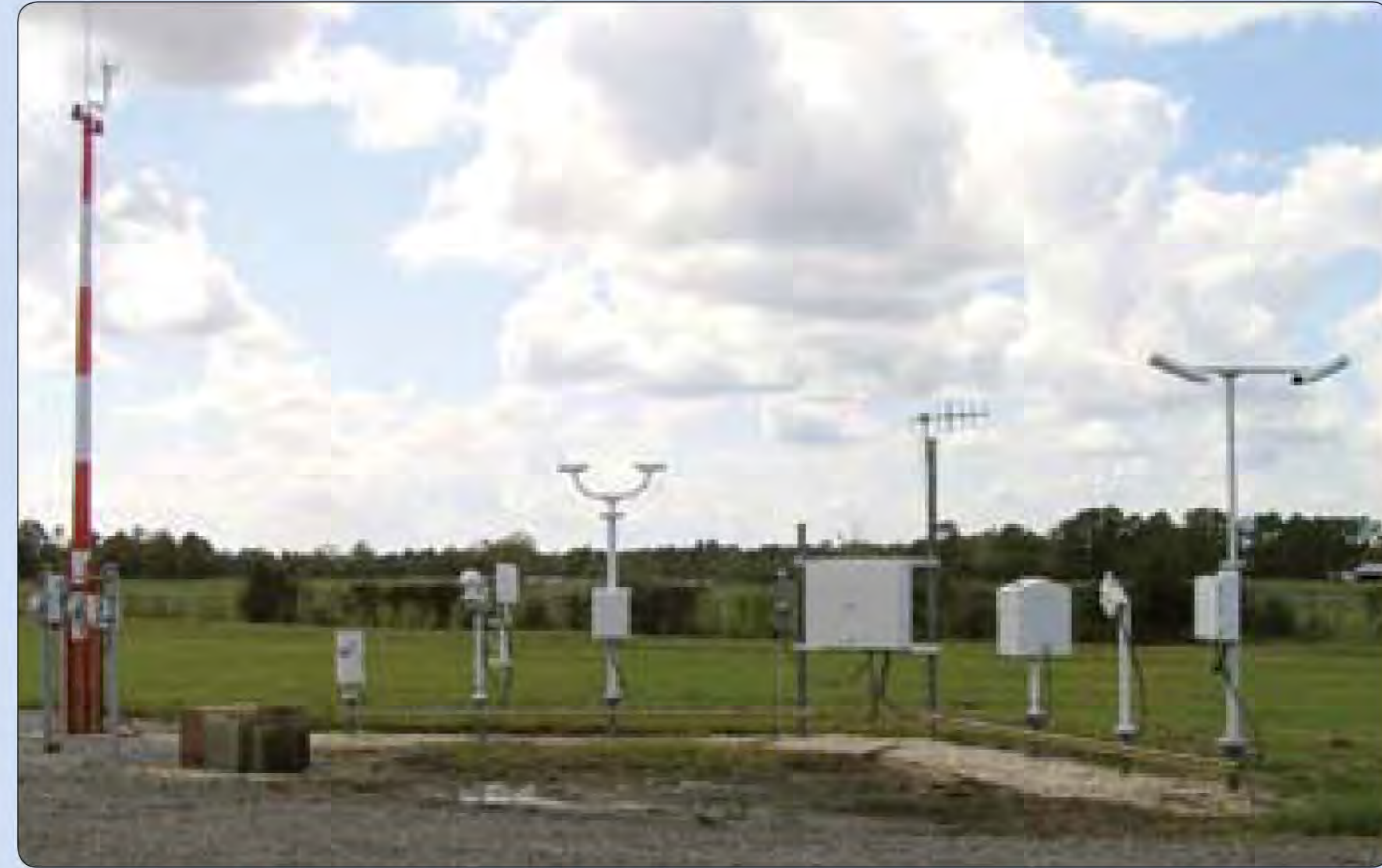
Above, the ASOS at the Morehead City, N.C., National Weather Service Forecast Office. Although the acronyms differ, an ASOS is functionally equivalent to the latest-configuration AWOS III-P-T.
