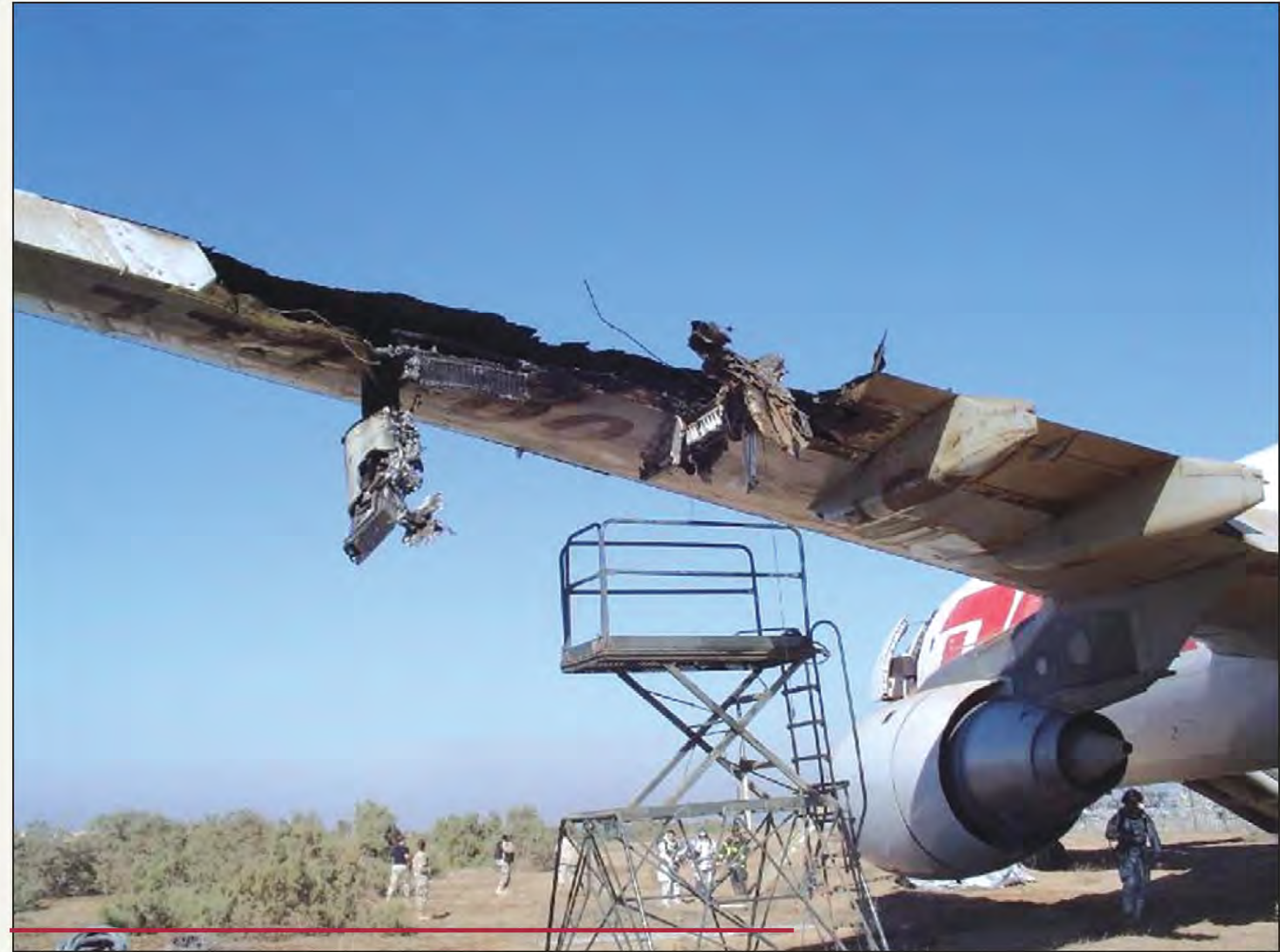
This DHL Airbus A300 was hit by a shoulder-launched missile while departing Baghdad, disabling all flight controls. Using only differential power, its crew was able to land and walk away.
