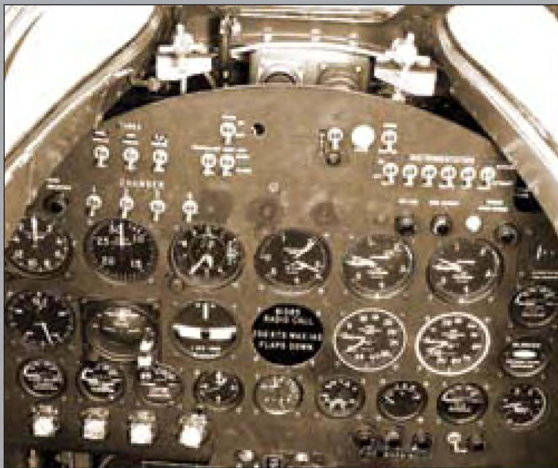
Top, a conventional turn-and-bank indicator. Bottom, the Bell X-1B's instrument panel is depicted, clearly showing the turn-and-bank instrument at left-center, with an artificial horizon next to it.
